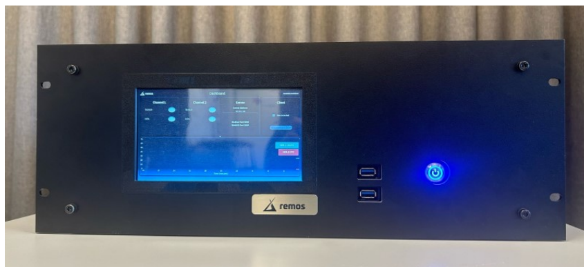
Figure 1: The front panel of the sequencer
